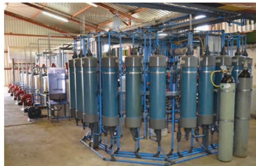
For treatment using the KNeW process, a twin line of stirred tank reactors (CSTRs) operate continuously, with the effluent water flowing from tank to tank. In the foreground is a ring of PLC controlled vessels for regenerating the resins: dilute nitric acid to regenerate the cation resin; and methanol for the anion resin.
